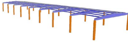
Figure 7: SAP2000 Structural Model
