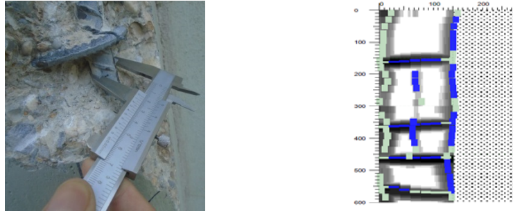
Figure 6. Identification of column reinforcement with clearing the cover and ferro-scan.
